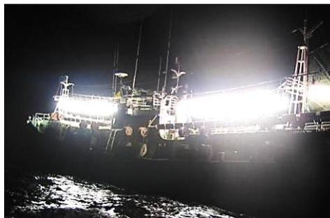
Gambar 10 Lampu pancing halida logam
