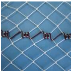
"Mountain" wrap joining (wrapped three times)
