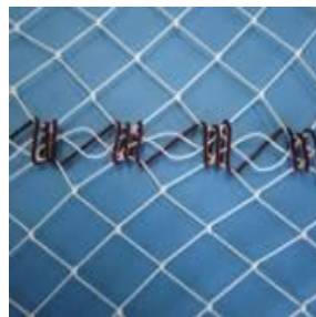
"Valley" wrap joining (wrapped three times)
