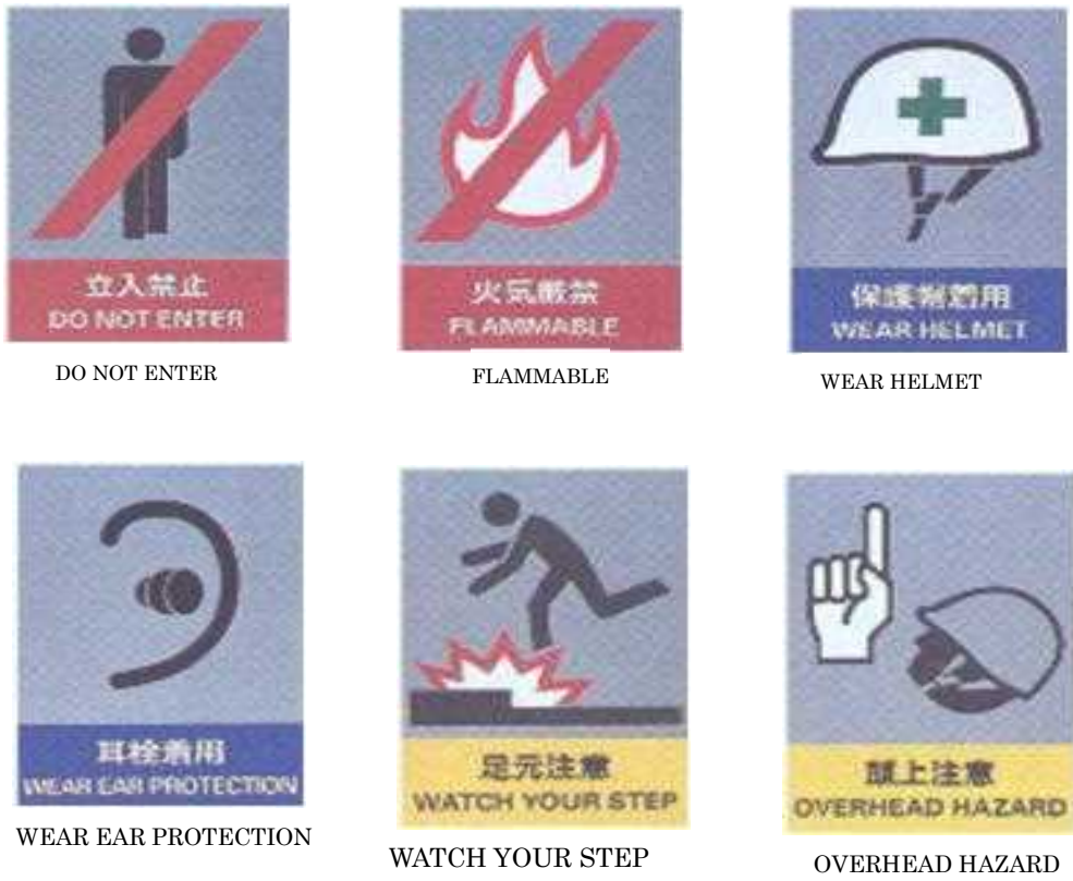
Figure 3: Examples of prohibition signs, instruction signs, and warning signs
